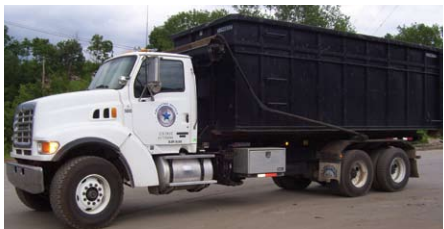
Above: An AMR "roll-off" truck used to pick up material onsite.
